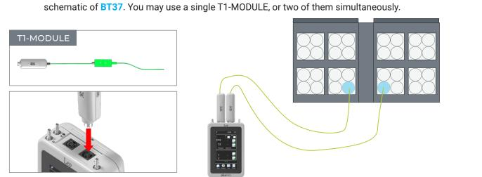
Place the cable of LEO's probe so that the tip of the sensor touches the bottom of the dish.
